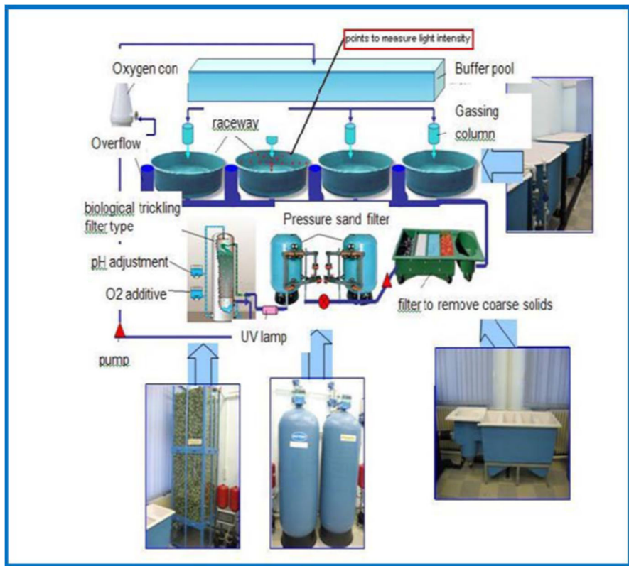
Figure 1. Pilot recirculation system configuration (Cristea V., 2008)
