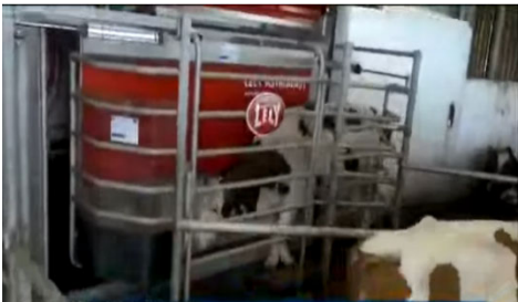
Fig. 2 Lely Astronaut milking robot (original photo)
