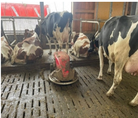
Fig. 4 Manure evacuation with the Lely Discovery robot (original photo)
