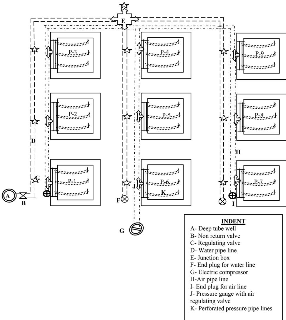
Fig-1. Schematic diagram of the experimental site
