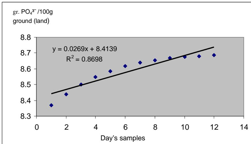
Figure No. 5. The Increase of the phosphorus content in recent sediments in the basin in the first eleven days after fertilization with super-phosphate, in the version with  $PO_4^{3-}$  1mg / l (second fertilization) ( $r = 0.93$ )
