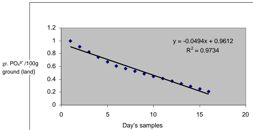
Fig. No. 7. The decrease of concentration of phosphate ions, after fertilization of the water basin with super Phosphate, nversion with 1mg/lPO<sub>4</sub><sup>3-</sup> (second fertilization)(r=0.98)
