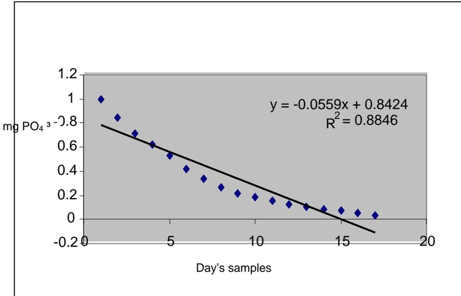
Figure No. 1. The dynamics Decrease of phosphate ion concentration, after fertilization of the water pond with super-phosphate, in version with 1 mg / l PO<sub>4</sub><sup>3-</sup> (fertilization First) (r = 0.94).
