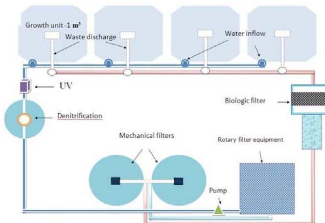
Fig. 1. The configuration of the experimental recirculating system.
