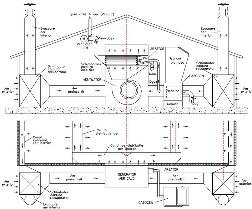
Fig. 1 Scheme of the installation of ventilation and heating with biomass
