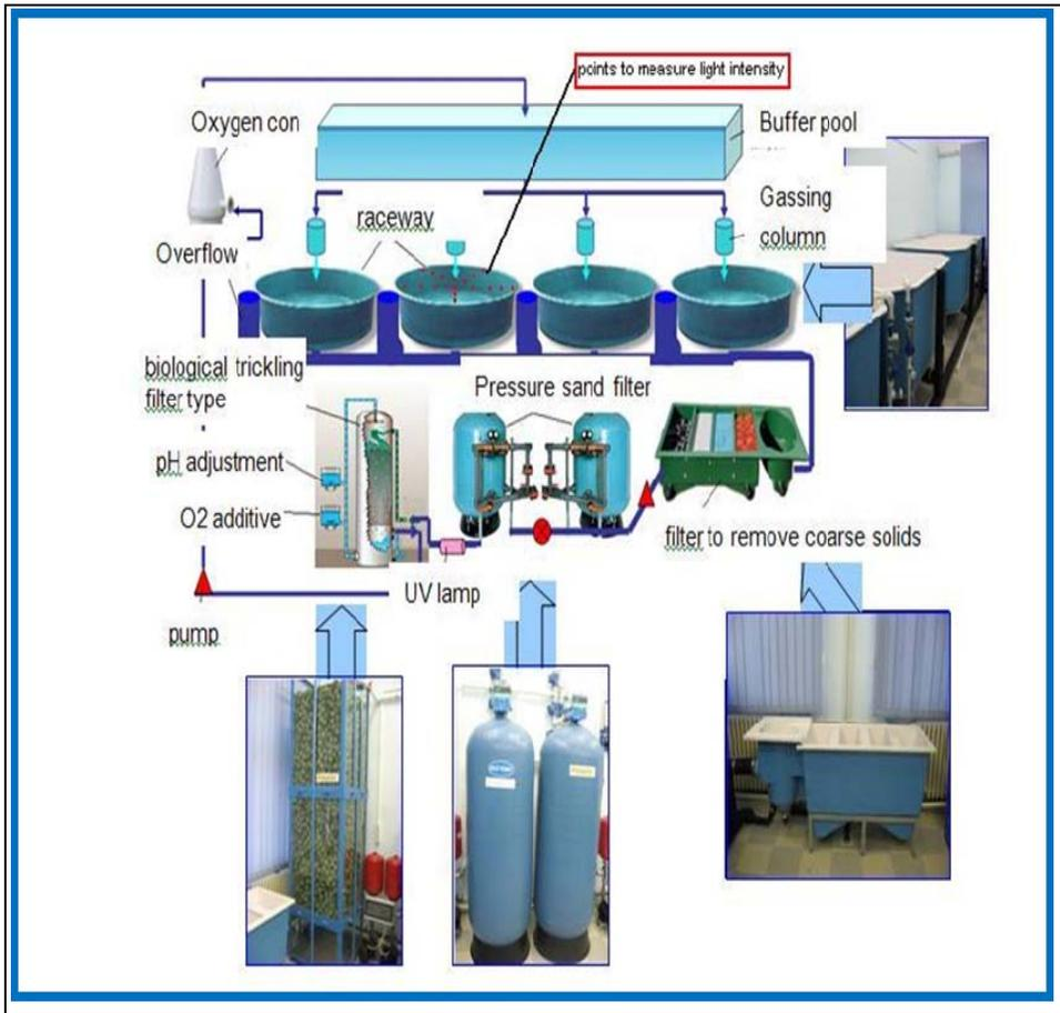
Figure 1 Recirculating system layout (Cristea, 2008)
