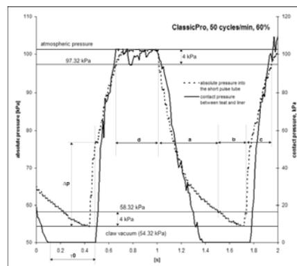
Fig. 4 Intermittent vacuum and contact pressure chart
