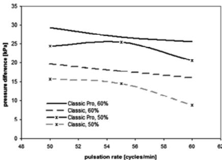
Fig. 6 The critical collapsing pressure difference
