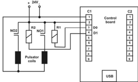
Fig.1 Schematics of the pulsator command circuit
