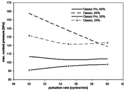
Fig. 5 The maximum teat-liner contact pressure
