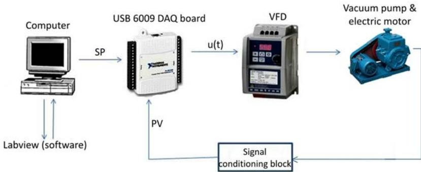
Fig. 5 The PID regulation loop
