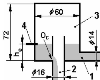
Fig. 1 The analyzed flowmeter drawing
