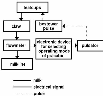
Fig. 2 Analyzed flowmeter location scheme
