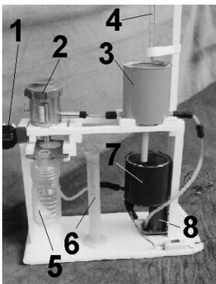
Fig. 3 Stand for measuring flow through the calibrated orifice flowmeter
