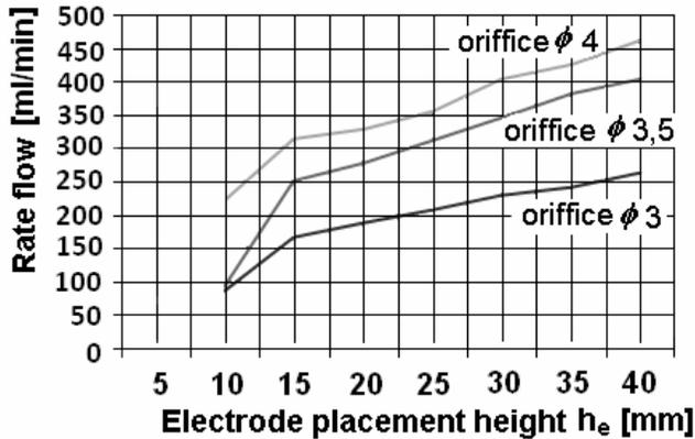
Fig. 4 Nomogram for choosing height placement of the electrodes
