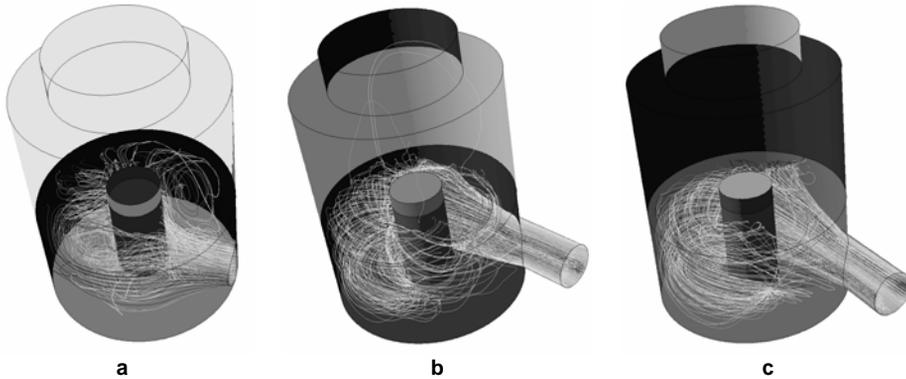
Fig. 5 CFD simulation of flow in the flowmeter
