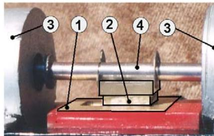
Figure 1 Operating parts of drawer type prototype pulsator
