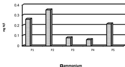
Fig. 4 Ammonium variation in experimental units - using zeolite as filter
