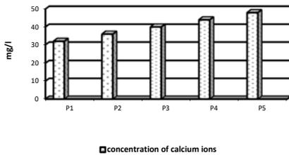
Fig. 8 Calcium ions variation in experimental units - using zeolite as filter
