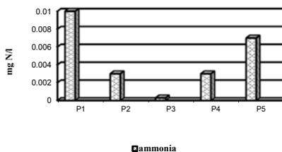
Fig. 3 Ammonia variation in experimental units - using zeolite as filter
