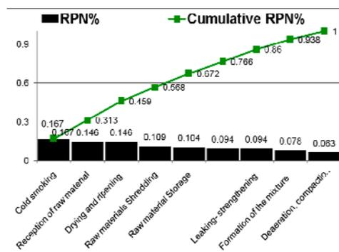
Fig. 2 Pareto Diagram for raw- dried salami before applying corrective action
