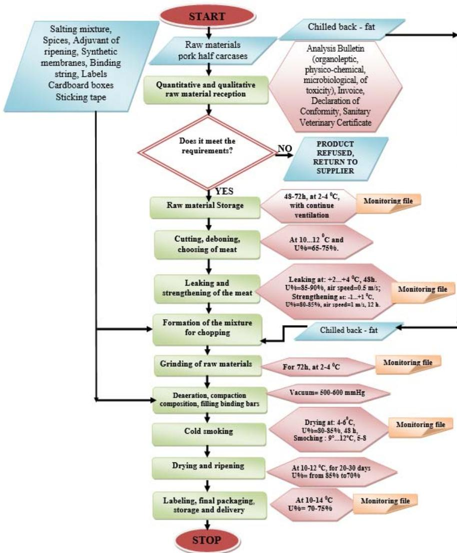
Fig. 1 The technological steps of raw-dried salami -adaptation after Banu et all, 2003 [6]
