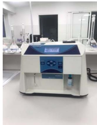
Fig. 5 Analizator EKOMILK-Spectra
