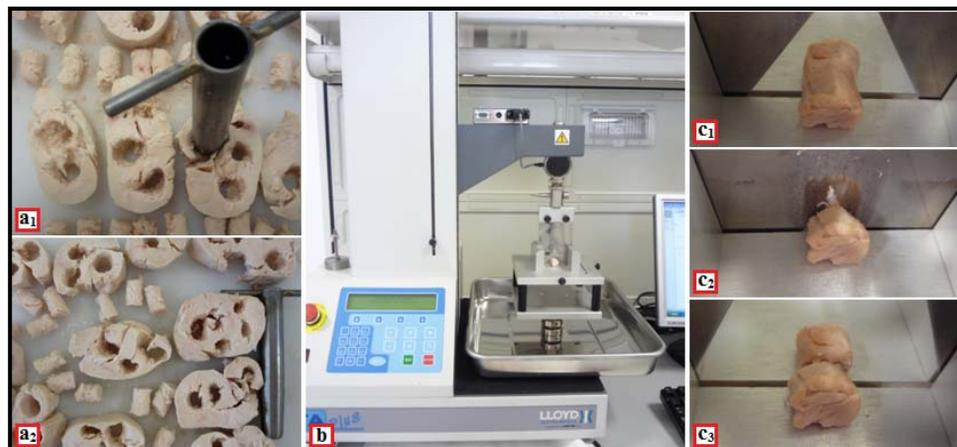
**Fig. 2**– Meat tenderness determination by using Warner Bratzel shear forces (a<sub>1</sub>, a<sub>2</sub> – cylindrically shaped cooked meat samples; b – determining performance; c<sub>1</sub>, c<sub>2</sub>, c<sub>3</sub> – successive stages of the V blade texture meter on the meat sample)
