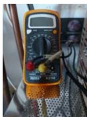
Fig. 5 NIMEX NI2100 Digital Multimeter
