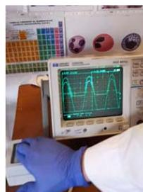
Fig. 16 Mono-alternating rectified AC on oscilloscope
