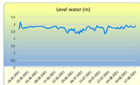
Fig. 4 Variation of level water in irrigation canal
