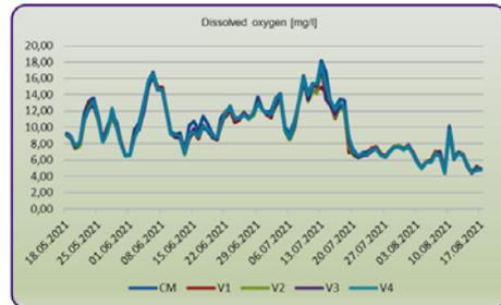
Fig. 3 Dynamics of dissolved oxygen in irrigation canal
