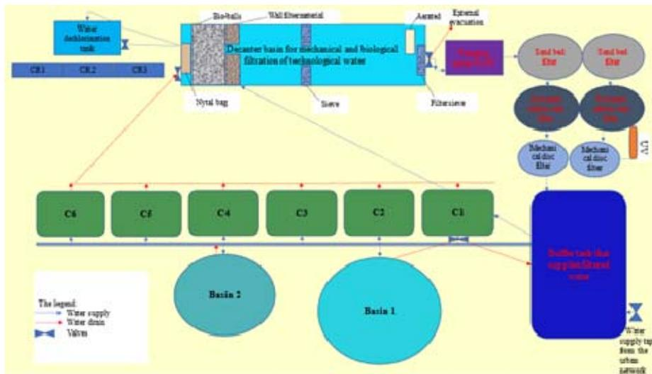
Fig. 1 Scheme of the recirculating aquaculture system.
