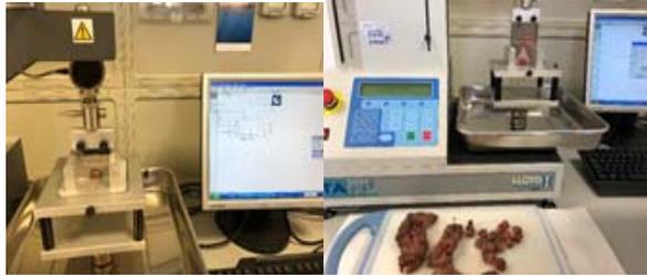
Fig. 3 Determination of Warner Bratzler forces
